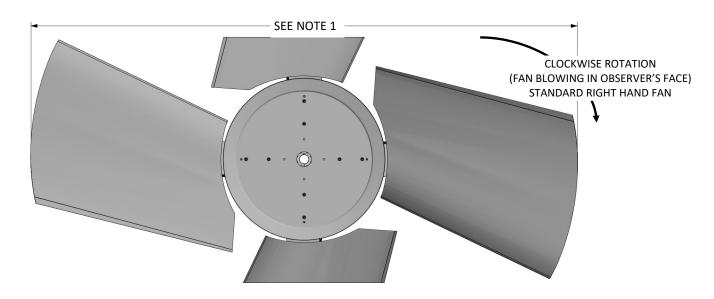
NOTE 1: MAXIMUM FAN DIAMETER EQUALS NOMINAL FAN DIAMETER. ADJUSTMENT OF  $\pm 1.5$  INCHES POSSIBLE AT INSTALLATION
