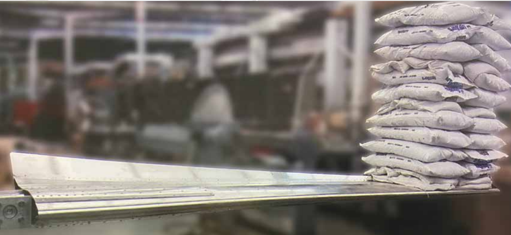
Lighter weight but supports 1,000 lbs at tips
