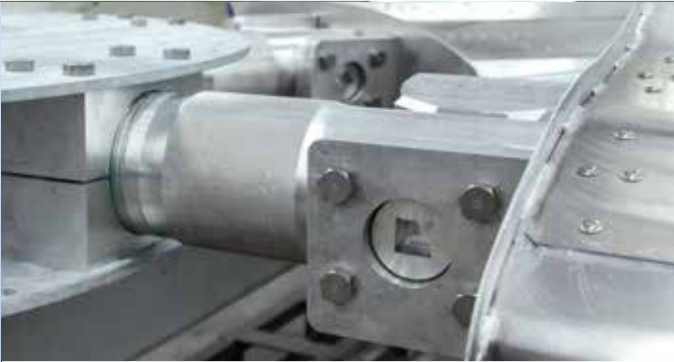
Adjustable diameter and blade angle
