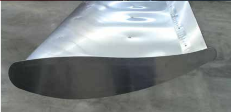
Vortex tips reduce noise and increase efficiency
