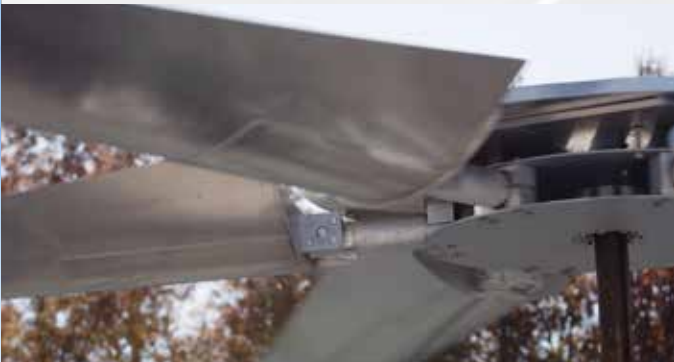
5052 marine grade aluminum blade
