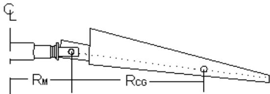
**The Solution:** In Moore fans, with the blades attached to the hub by a resilient mount, or pivot, this
