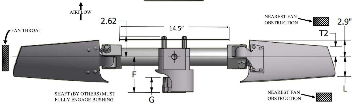
SHAFT (BY OTHERS) MUST FULLY ENGAGE BUSHING
