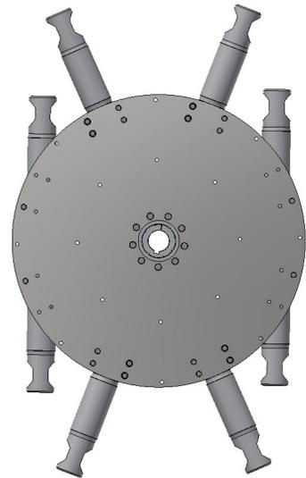
The hub requires rod ends / blocks pivoted into place.
