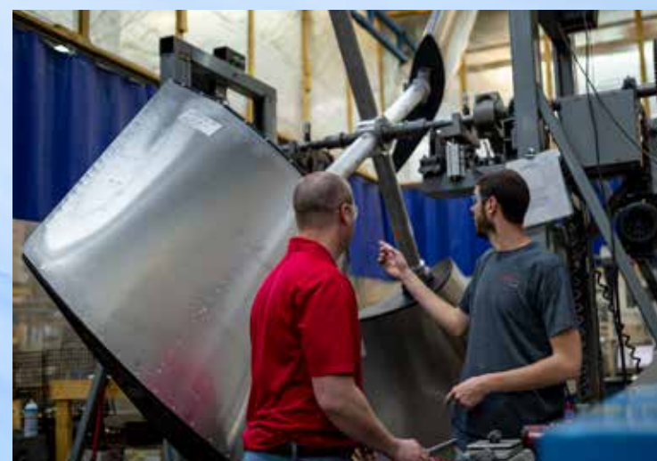
MAG fan being balanced for precision performance
